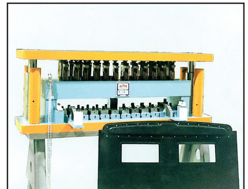
Tog-L-Loc® "bump" die for joining pre-painted aluminum sunroof.
