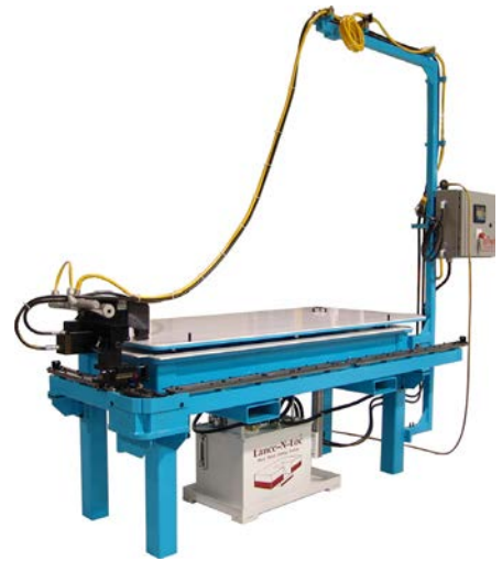
This custom solution uses a BTM 7007 hand-held unit, fixed to a track to easily clinch various locations of a part.
